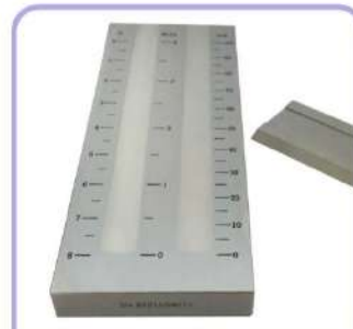
刮板细度计/双槽 Fineness of Grind Gauge/Double Groove
