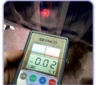
SIMCO静电场测量仪FMX004 Electrostatic field measuring instrument
