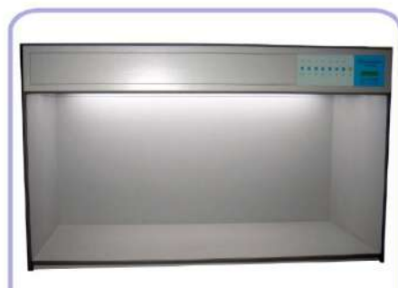
标准光源对色灯箱CAC-1200L Standard light source color light box
