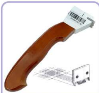
漆膜划格器/单面 Cross Cut Tester/Single side
