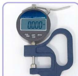
数显测厚规0.001mm 0~12.7mm Digital thickness gauge
